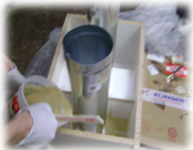
Liquid Foam being poured
